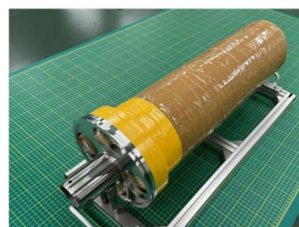
Membrane element ( \phi = 20 cm; L = 60 cm)
